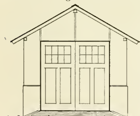
FIGURE FOUR: FRONT ELEVATION OF GARAGE SHOWING METAL COVERED DOORS, CONCRETE FOUNDATION WALL, AND PANELS OF "TRANSITE ASBESTOS LUMBER" ABOVE WITH BATTEN STRIPS OVER JOINTS.
